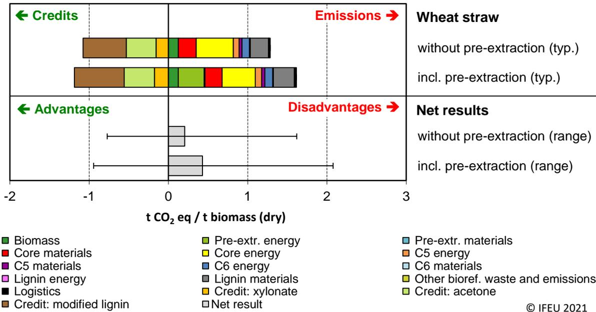
Figure 18: Comparison of life cycle greenhouse gas emissions of the UNRAVEL biorefinery using wheat straw as biomass feedstock without and including a pre-extraction process preceding the core process. Error bars indicate the range from optimistic to conservative.
