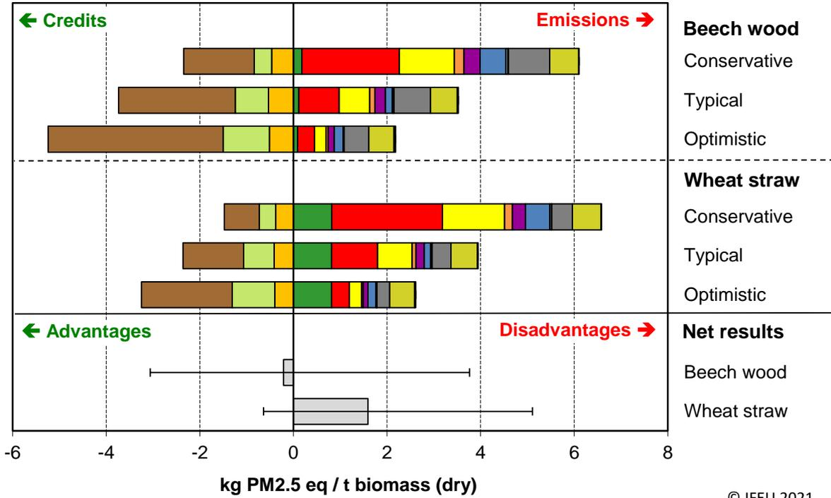
Figure 40: Particulate matter formation of the basic scenario (beech wood) and the scenario on wheat straw use without pre-extraction under typical, conservative and optimistic boundary conditions.
