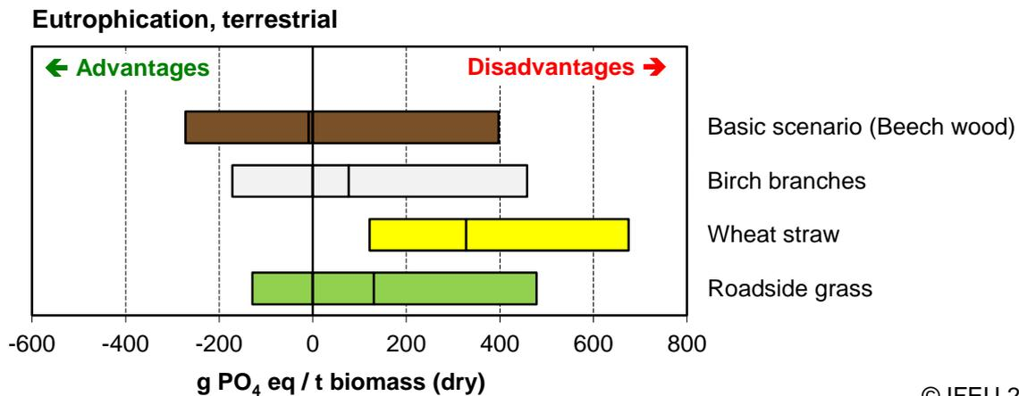
Figure 17: Comparison of terrestrial eutrophication of various scenarios of the UNRAVEL biorefinery using different feedstocks.
