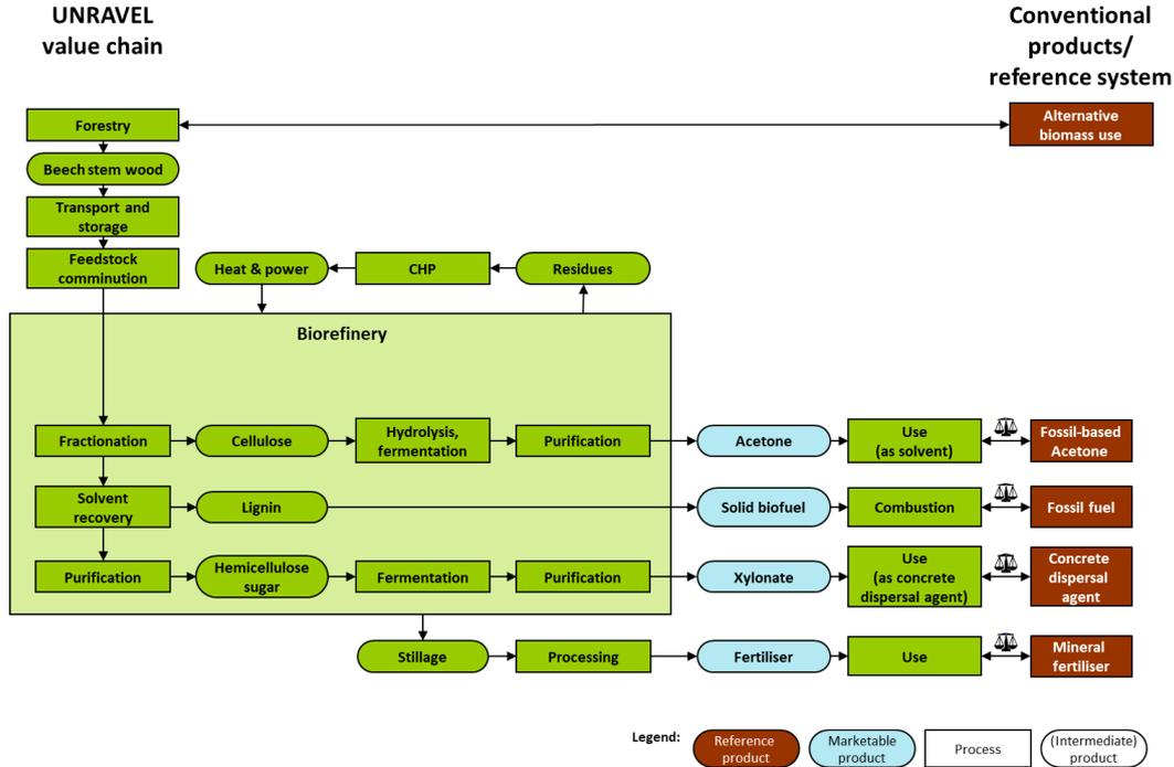
Figure 24: Life cycle scheme of the scenario 'lignin combustion'.
