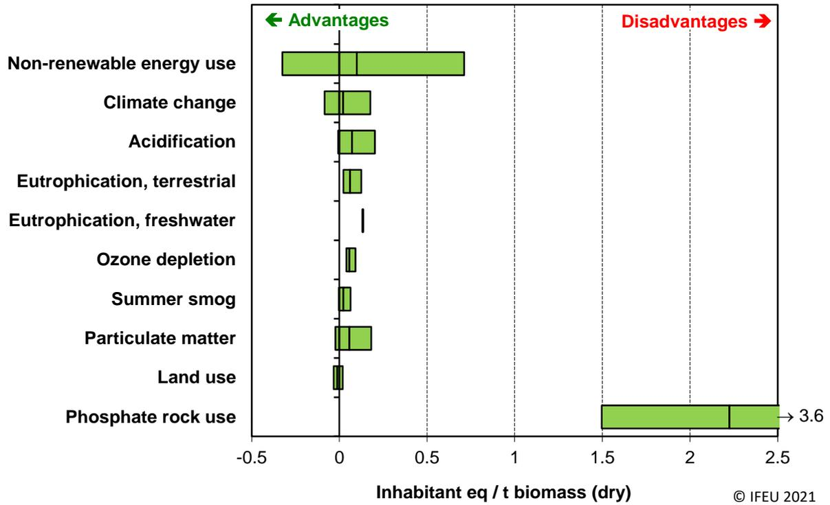
Figure 43: Normalised LCA results (in inhabitant equivalents) of the scenario on wheat straw use without pre-extraction for all impact categories. The bars show the results under a range of possible boundary conditions primarily relating to technology development.
