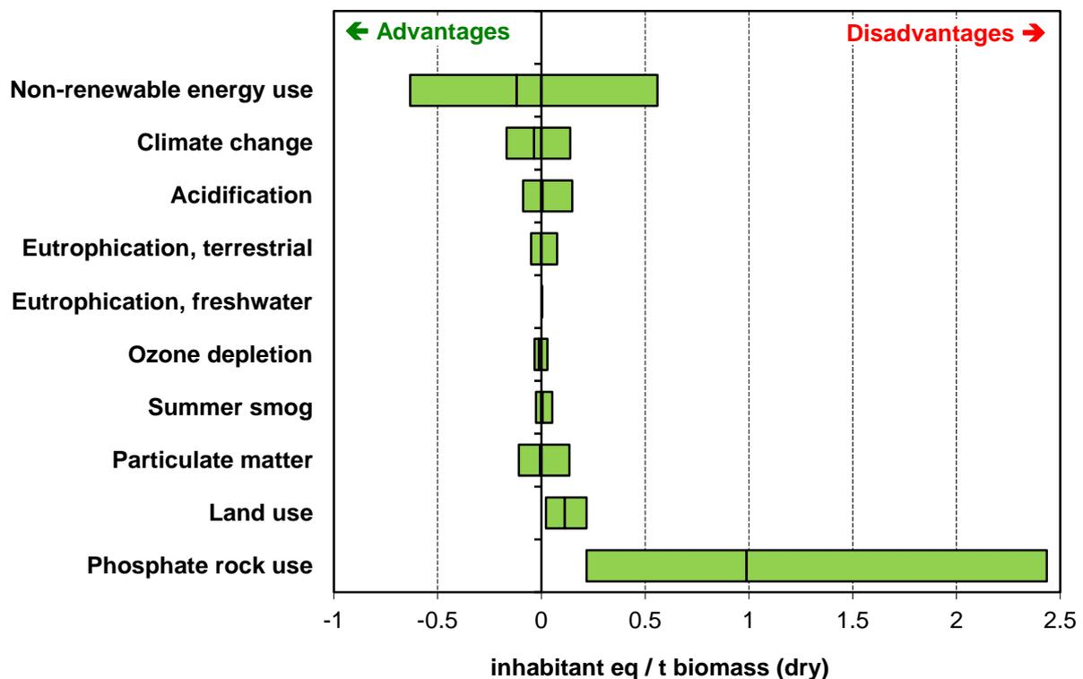
Figure 12: Normalised LCA results (given in inhabitant equivalents) of the basic scenario (beech wood) compared to its reference products for all analysed impact categories. The bars show the results under a range of possible boundary conditions from optimistic via typical to conservative primarily relating to technology development.
