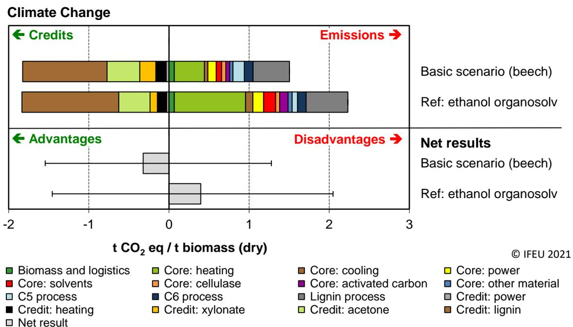
Figure 13: Comparison of life cycle greenhouse gas emissions of the basic scenario using the Fabiola process (acetone organosolv) with those of the reference scenario using the conventional ethanol organosolv process. Error bars indicate the range from optimistic to conservative.
