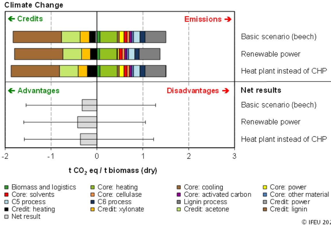
Figure 14: Comparison of life cycle greenhouse gas emissions of the basic scenario (using fossil and renewable power<sup>1</sup>) and using a heat plant instead of a combined heat and power plant (CHP). Error bars indicate the range from optimistic to conservative.
