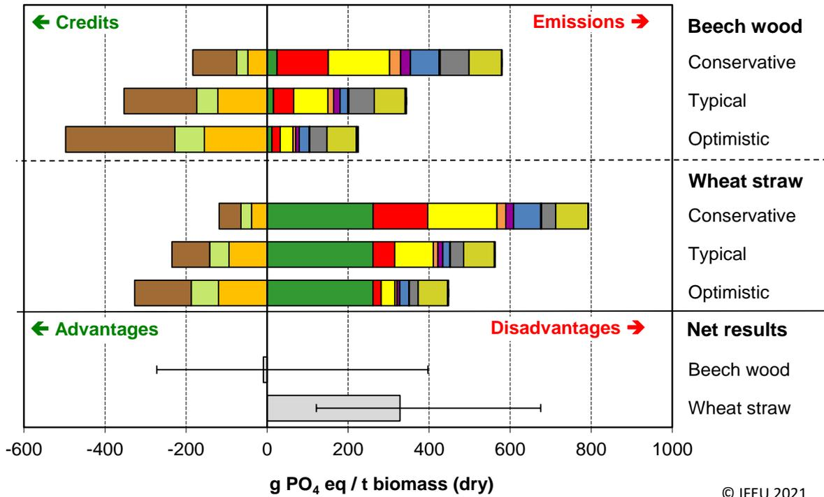
Figure 36: Terrestrial eutrophication potential of the basic scenario (beech wood) and the scenario on wheat straw use without pre-extraction under typical, conservative and optimistic boundary conditions.
