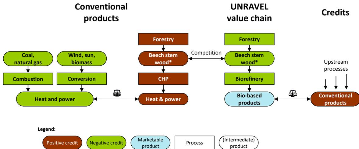
Figure 9: Life cycle scheme of the beech wood scenario including the competing use of beech stem wood\* for energy in a combined heat and power plant. \*Quality: energy/pulp wood.
