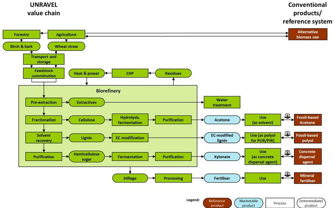
Figure 32: Life cycle scheme of the scenario 'physically mixed feedstock'.
