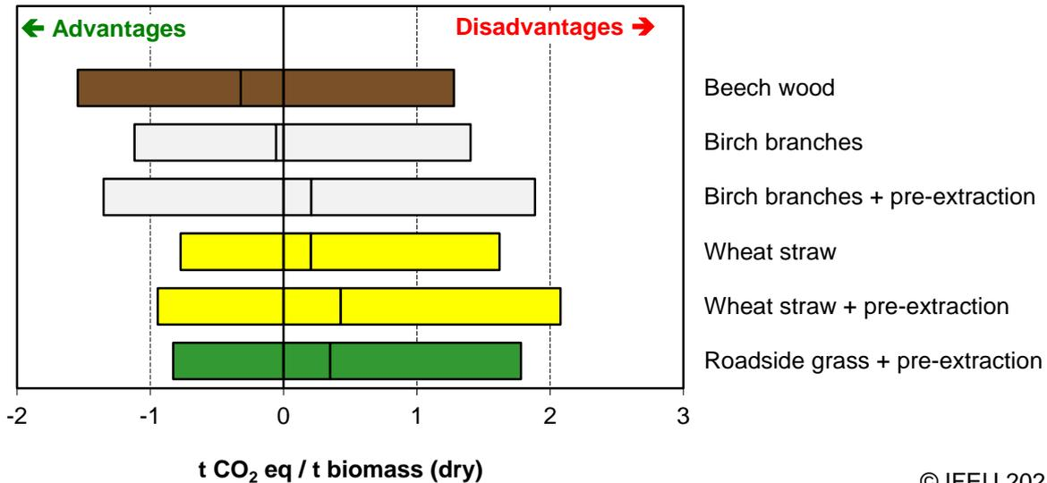
Figure 19: Comparison of life cycle greenhouse gas emissions of various scenarios of the UNRAVEL biorefinery using different feedstocks without/including a pre-extraction process.
